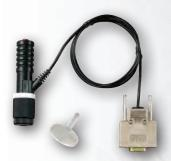
Order No. **810-288-10 Model : UD-412 DC type**Use for inner walls of cylinders.
