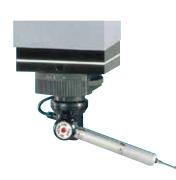
PH1 is a manual positioning probe head that allows positioning at the horizontal surface rotation angle of  $360^{\circ}$  ( $15^{\circ}$  pitch) and vertical surface rotation angle of  $\pm 115^{\circ}$ .
