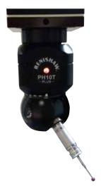
PH10T PLUS is a motorized indexing probe head whose horizontal surface rotation angle is  $\pm 180^{\circ}$  and whose vertical surface rotation angle is 0 to  $\pm 105^{\circ}$ . It allows positioning at a pitch of 7.5° in both directions.
