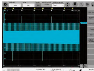
Continuous acquisition with no blind time
