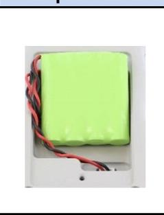
You can open the battery cover of DSV/DST, and replace it very easily.
