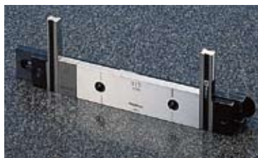
Use of B-type connectors in gage construction
