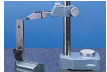
Setting a dial test indicator to a long-gauge-block stack attached to the base with a D-type connector
