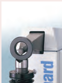
The dolphin-nose indenter arm for inside testing
