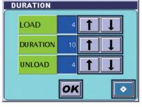
In addition to the test force dwell time, you can specify loading and unloading testing actions.
