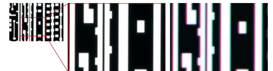
Apochromat optics (captured with SMZ1270+Plan Apo 1x/WF)
