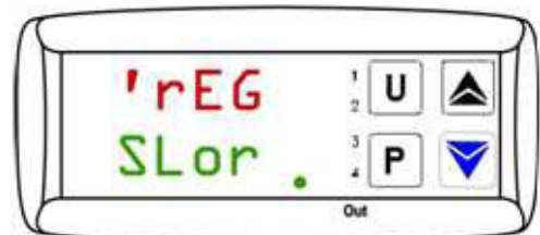
Parameters for heating gradient SLor
