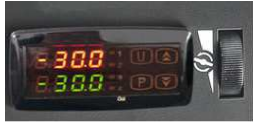
Front of the controller with stirring speed wheel
